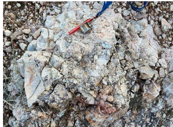
Map of the Bottom-Up target area displaying alunite, kaolinite, and illite hyperspectral results with arsenic in soil samples. Photos of outcrop demonstrate strong silicification and local veining and brecciation
