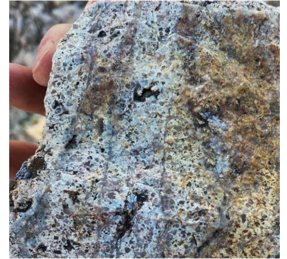
Map of the Bottom-Up target area displaying alunite, kaolinite, and illite hyperspectral results with arsenic in soil samples. Photos of outcrop demonstrate strong silicification and local veining and brecciation
